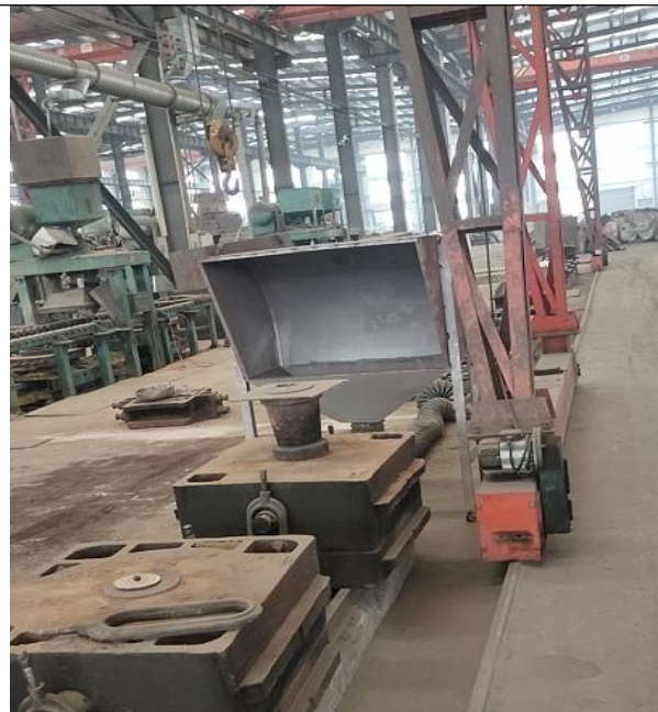
覆膜砂浇注废气移动式集气罩
